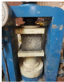
Fig1 Testing of cube in UTM machine
